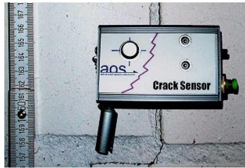
b) More compact model of a crack sensor applied over a vertical crack (MBC Dr. B. Mueller, Leipzig, Germany).
